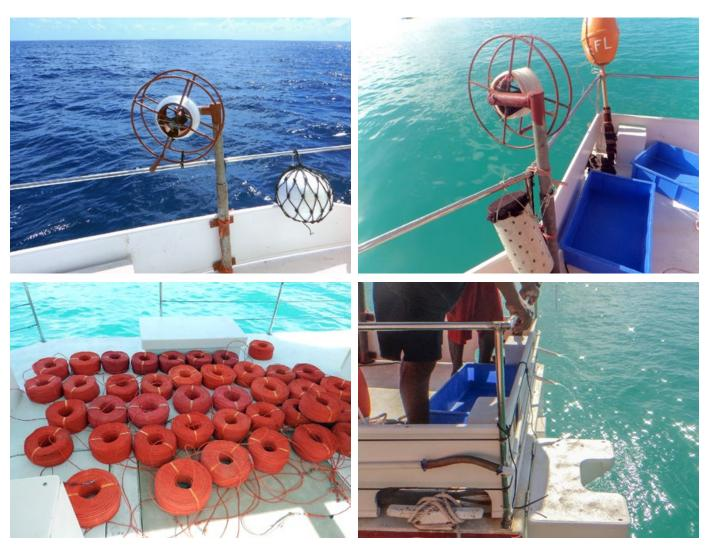
Top left: Metal handreel to facilitate trolling and midwater fishing. Top right: A chum bait canister hanging beside the handreel ready for use. Bottom left: Kuralon rope as mainline. Bottom right: Spray system installed for dangler fishing.
