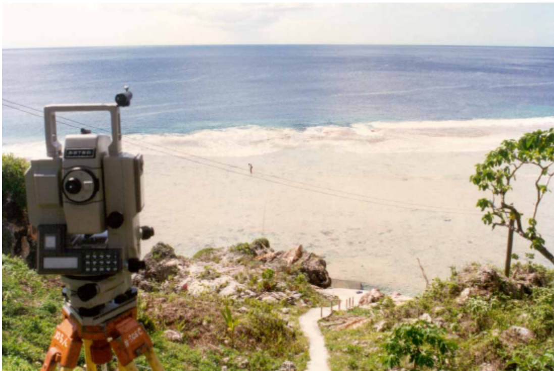
Figure 22. Tuapa Landing from top of sea track, with Sokkia Set 2C total station survey instrument in foreground. Chainman Sione Tongiakona, carrying the survey target, is halfway across the reef platform in the distance. (DLF/ 7 Nov 1995).
