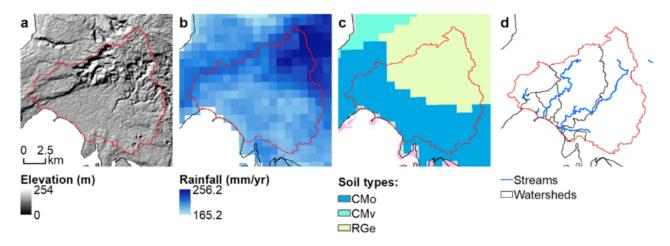
Fig S2. Terrestrial geography & InVEST SDR inputs. (a) Digital Elevation Model (DEM), (b) average yearly rainfall (mm/yr), (c) soil types, (d) streams and watershed boundaries within the area of interest.
