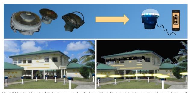
Figure 3. Mata Utu high school students re-purposed washed-up dFAD satellite buoys into autonomous outdoor solar lamps for the main entry of the school, or used as phone chargers. (images: @Mata Utu High School)
