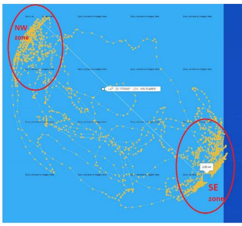
Figure 3. Two months of FAD surface float positions (yellow dots), showing two main trends in relation to the estimated FAD anchor position: a southeast zone when the nearshore oceanographic current actively pushes towards this direction; and a northwest zone when the oceanographic current ceases and the usual southeast trade winds are active, pushing the mooring line towards the northwest.
