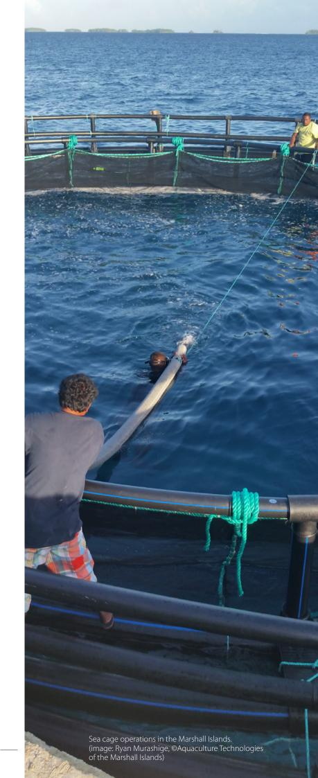
Sea cages are generally moored in a grid system designed to dampen the forces of weather. The longitudinal axis of the grid is positioned across the direction of greatest wave action and current flow in order to maximize water exchange; routinely, a minimum depth of 10 m or so is required. A properly moored sea cage marine farm can withstand wind speeds of up to 150 km/hr.
