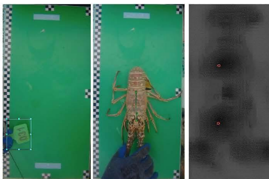
Figure 3. Automated object identification (tag for traceability; left), annotated lobster (center), and the heat map (right) of automated lobster carapace measurement.
