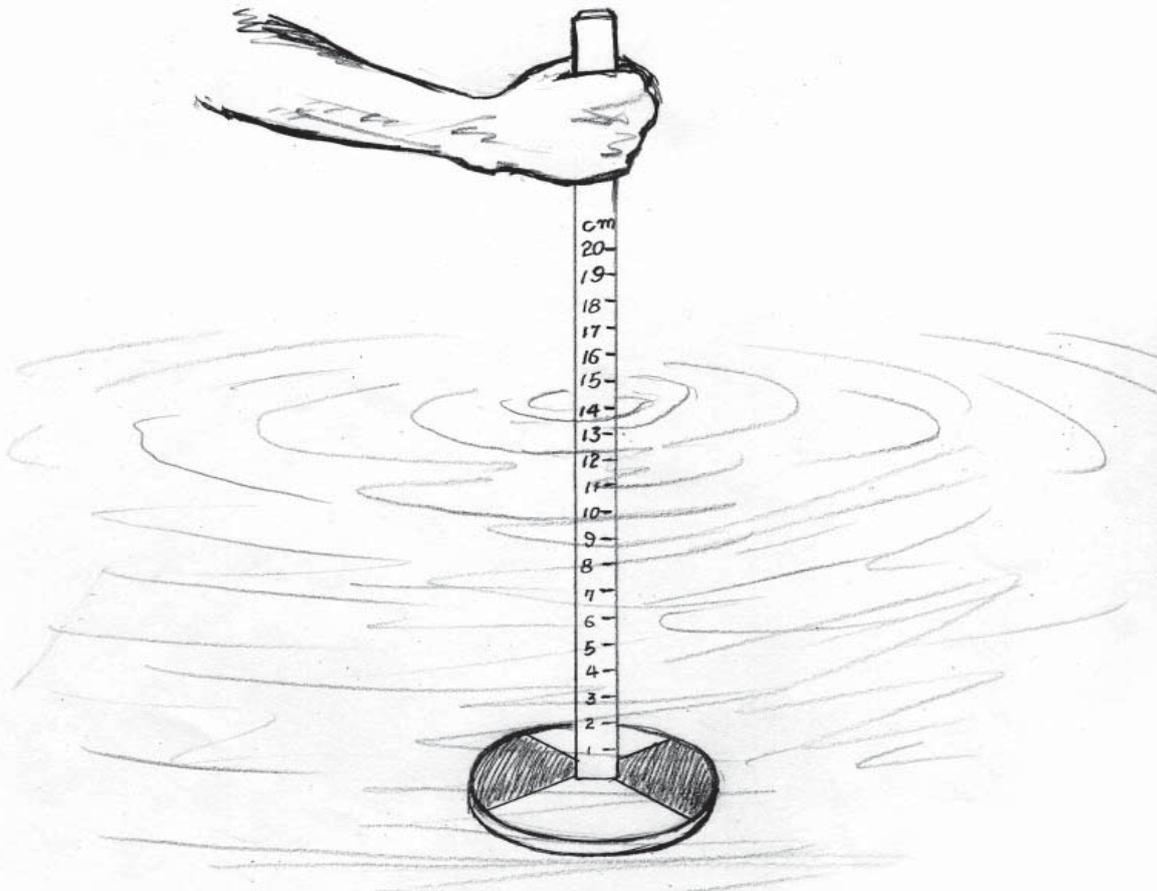
Figure 16. Measuring water transparency with a Secchi disc
