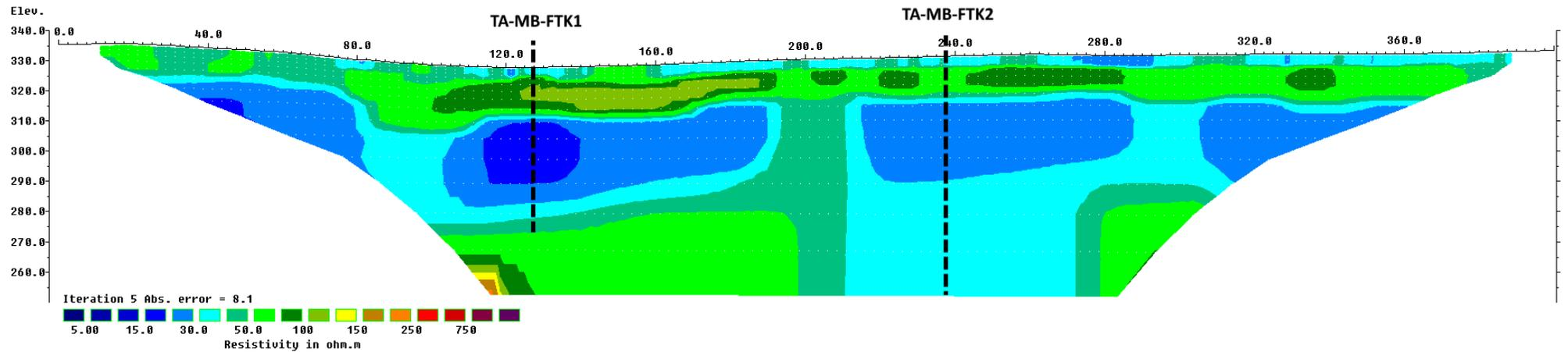
Figure A12. Resistivity profile and proposed drilling targets along survey line 12 (Fetukai).
