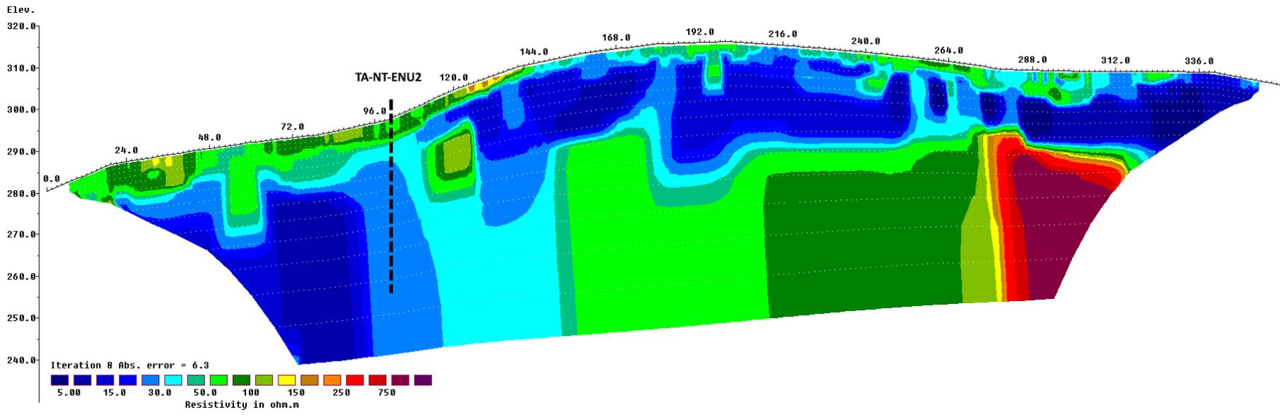
Figure A4. Resistivity profile and proposed drilling targets along survey line 4 (Ehniu 2).
