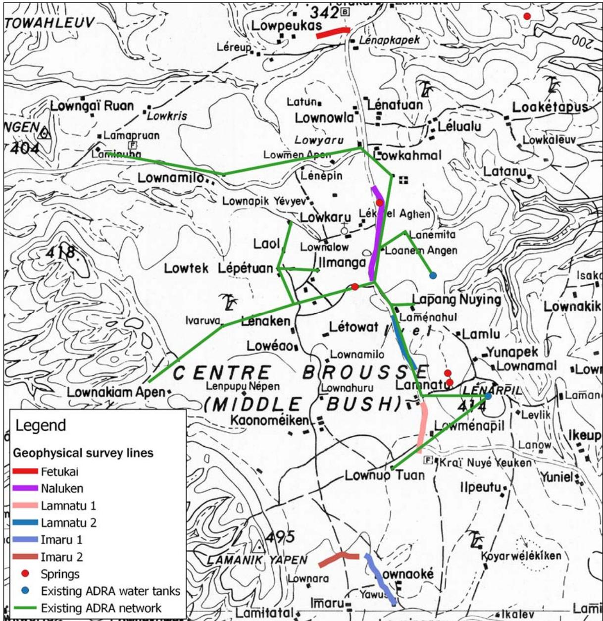
Figure 2. Adventist Development and Relief Agency (ADRA) water pipeline connecting water tanks with communities. In reality, the network is only able to serve communities at close proximity to the Lenarpil water tanks with the current water supply.
