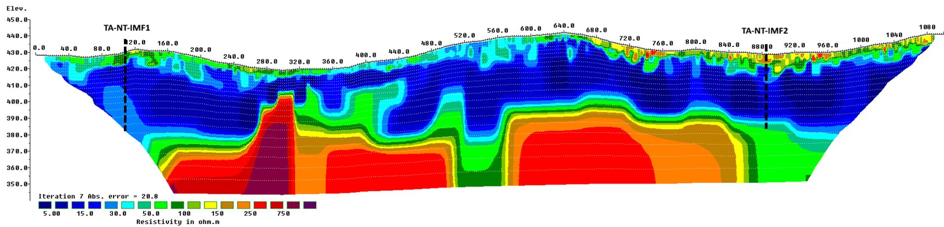
Figure A2. Resistivity profile and proposed drilling targets along survey line 2 (Lownimhapon – Imafin).
