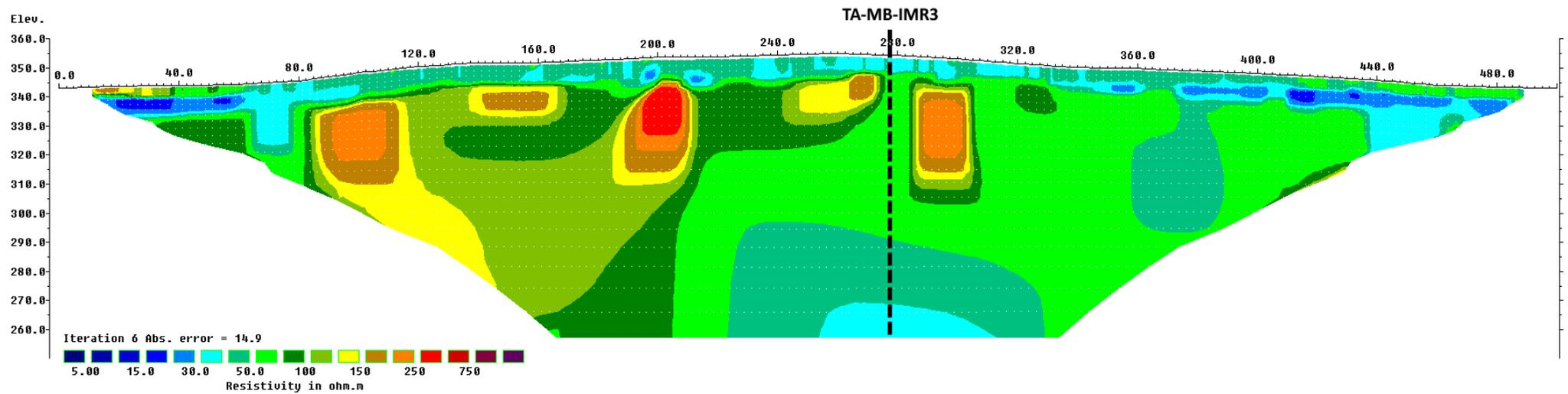
Figure A8. Resistivity profile along survey line 8 (Imaru 2).
