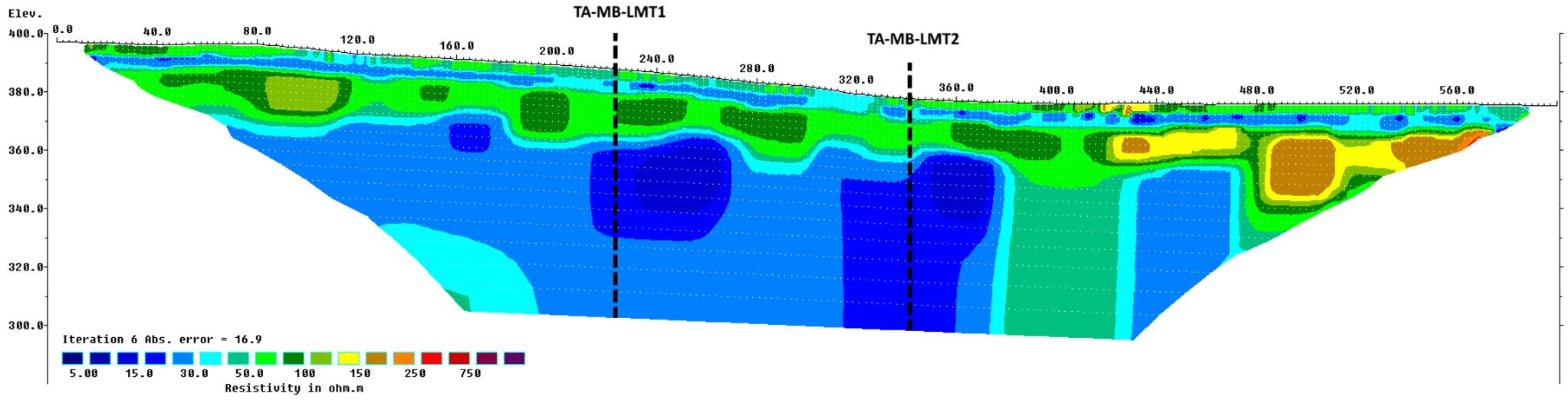
Figure A9. Resistivity profile and proposed drilling targets along survey line 9 (Lamnatu 1).
