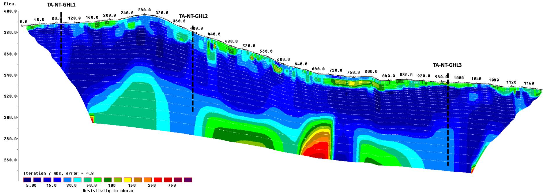
Figure A1. Resistivity profile and proposed drilling targets along survey line 1 (Lownaleng – Green Hill).
