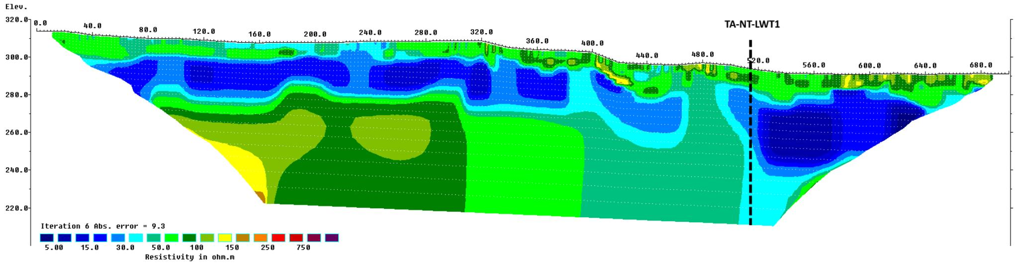
Figure A5. Resistivity profile and proposed drilling targets along survey line 5 (Lawital).
