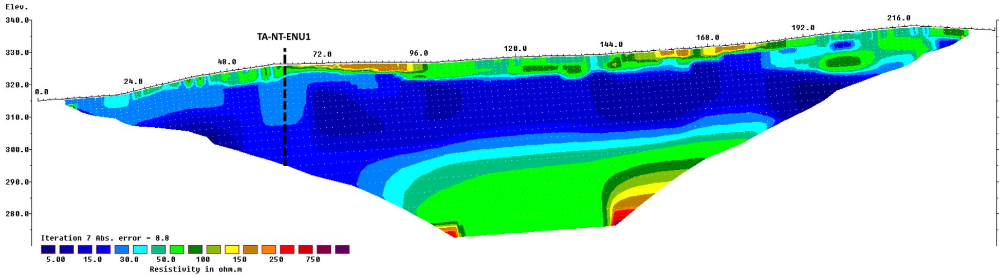
Figure A3. Resistivity profile along survey line 3 (Ehniu 1).
