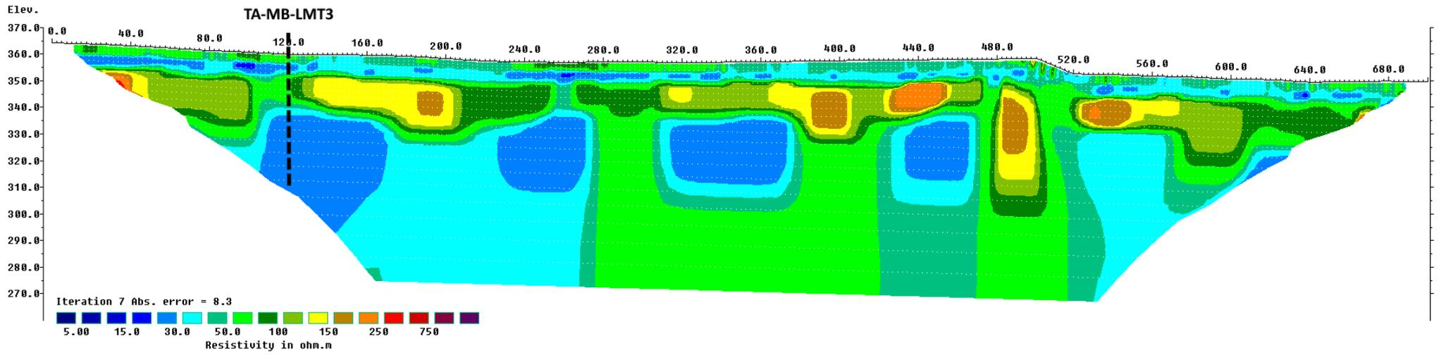
Figure A10. Resistivity profile and proposed drilling targets along survey line 10 (Lamnatu 2).
