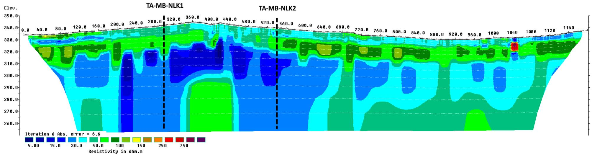
Figure A11. Resistivity profile and proposed drilling targets along survey line 11 (Naluken).
