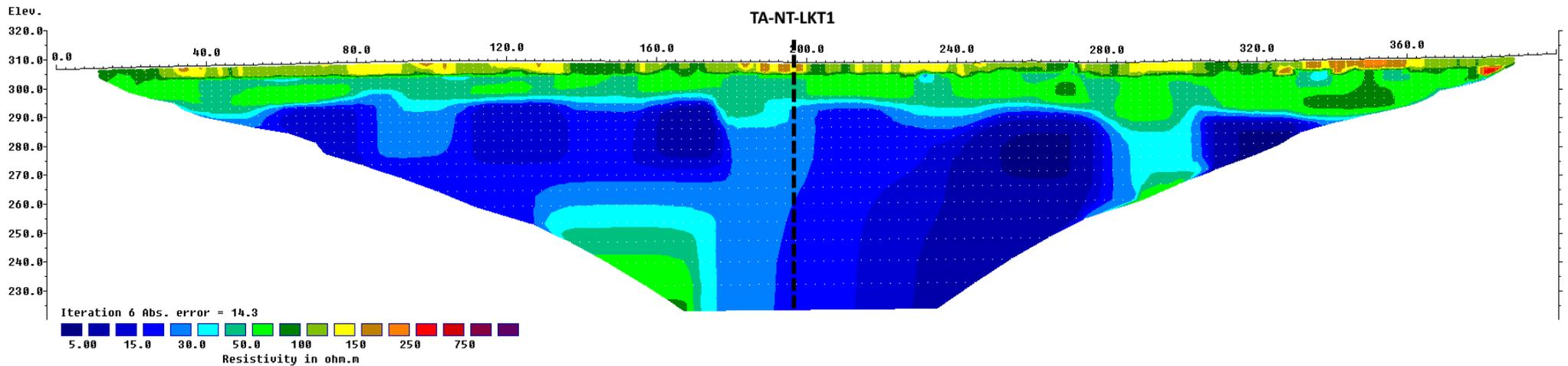
Figure A6. Resistivity profile and proposed drilling targets along survey line 6 (Laketam).
