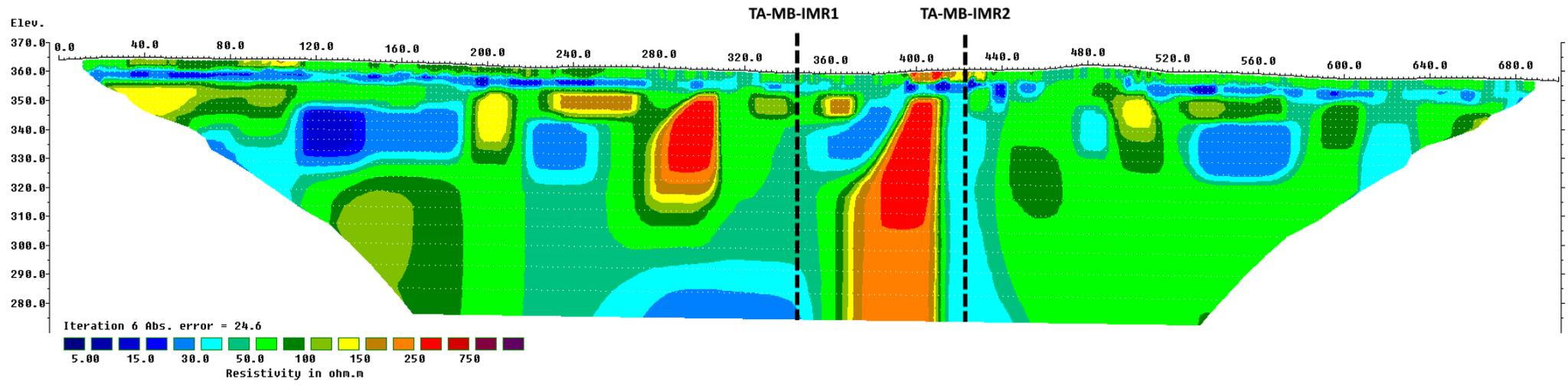
Figure A7. Resistivity profile and proposed drilling targets along survey line 7 (Imaru 1).
