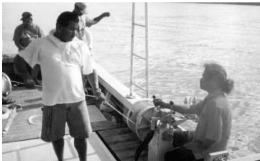
Figure 4: Vertical longline hauler on F/V Elechil
