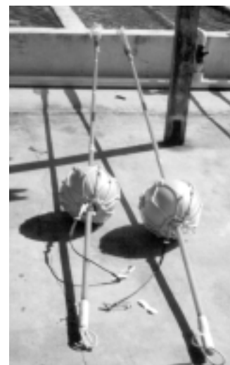
Figure 10: Flag buoys made up with strobe lights attached
