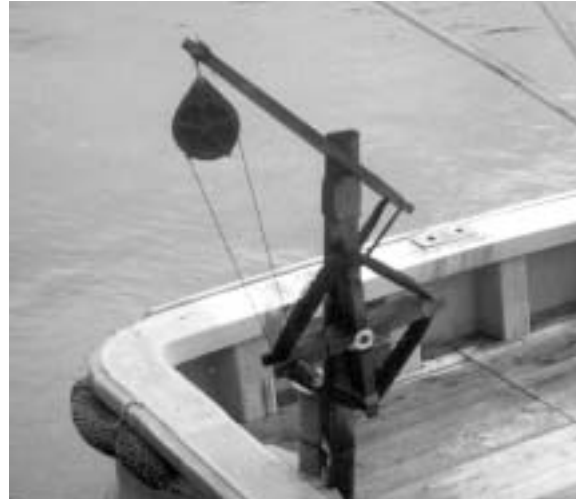
Figure 8: Palu-ahi line stored on a wooden handreel
