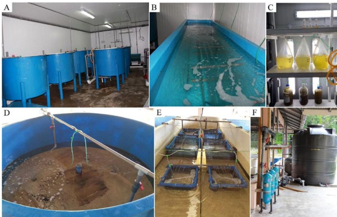
**Figure 1.** Sea cucumber rearing facilities. A: Hatchery unit with larval culture tanks; B: Indoor nursery tank with settlement plates; C: Phytoplankton room with *Chaetoceros* sp. cultures; D and E: Outdoor nursery tanks holding juveniles > 10 mm in size; F: Seawater storage and filtration system.
