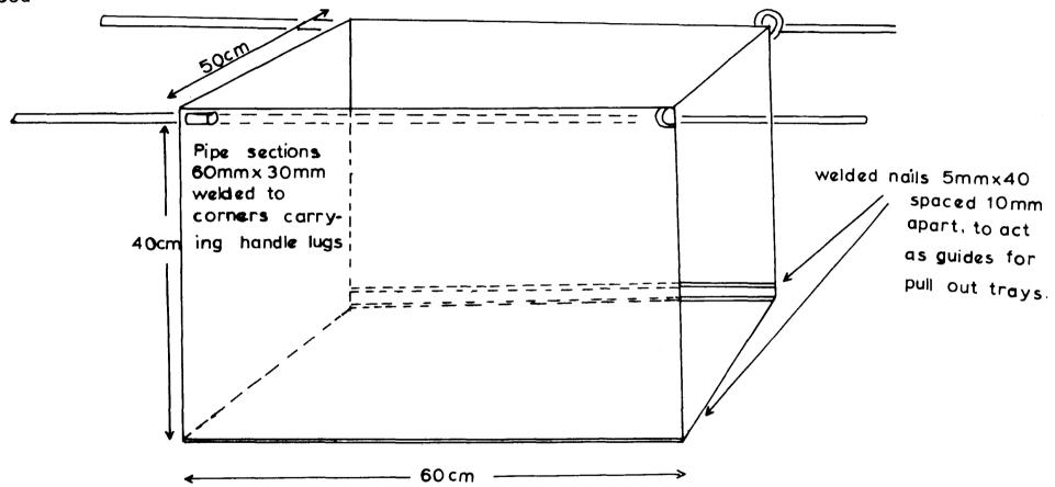
Container consists of 4 sided steel box, welded out of 4mm sheet, with open top & separate sliding bottom tray running on guide nails welded longitudinally along inside bottom lip. Tray was 5mm sheet with rouded off corners usually had to hammered home in order to cut through sand blocking the guide nails.
