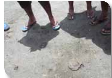
Figure 85. Drop the ball to the ground from head height. If it shatters or crumbles, the soil is too sandy to be water tight. If it stays together, as shown, the clay content is sufficient to stop water leaking out.
