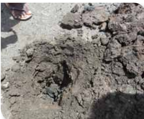
Figure 86. Another leak test can be performed by digging a hole down to where the bottom will be. Fill the hole with some water and mark its level. If the water drains out within a couple of hours, then the soil is too sandy.
