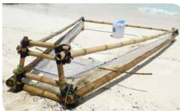
Figure 32. An alternative style of construction, using 100% bamboo (no timber). Strips of car tyre inner-tube instead of rope for lashing enables much faster assembly and disassembly for carrying the bulldozer net to different sites in a vehicle or boat.
