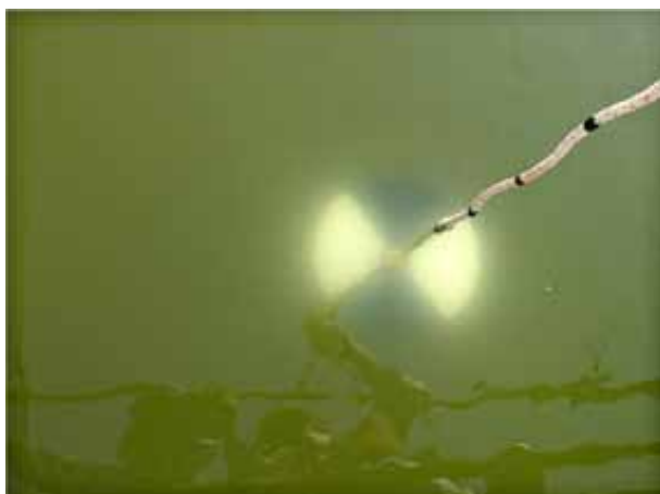
Figure 17. When the black&white zone of the secchi disk just disappears from view when lowered into the pond water, read off the secchi value in cm from the graduations marked on the rope
