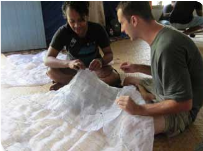
Figure 39. Re-inforcing the double-layer cod-end with additional seams. The double layer of mesh reduces the pressure of water current forcing fry up against the net, thus reducing injury and mortality.
