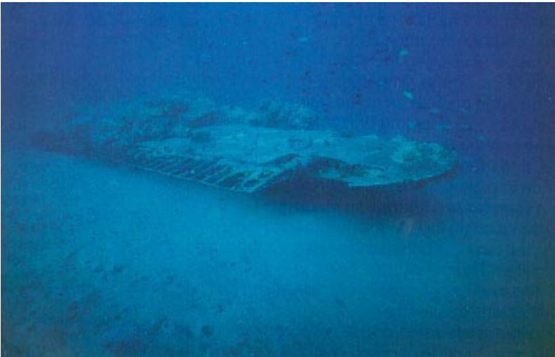
Plate 17. Underwater photograph of a submarine in Iron Bottom Sound. Note the heavily encrusted and highly corroded metal surface. Encrustation of various types of marine algae and small corals are common. Photo reproduced with the kind courtesy Solomon Islands Visitors Bureau, Ministry of Tourism, Honiara.
