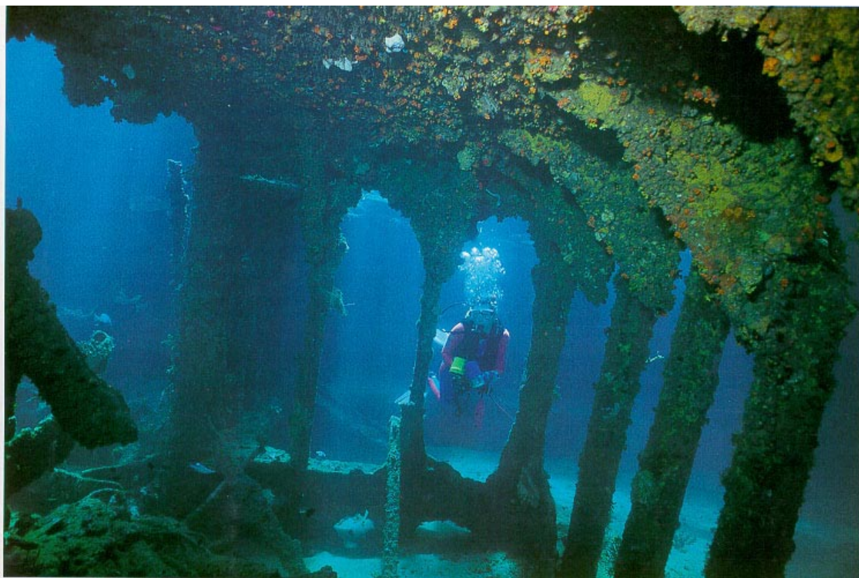
Plate 12. Underwater photograph of a battleship in Iron Bottom Sound. Note the heavily encrusted and highly corroded metal surface. Encrustation of various types of marine algae and small corals are common. Photo reproduced with the kind courtesy Solomon Islands Visitors Bureau, Ministry of Tourism, Honiara.
