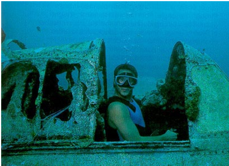
Plate 19. Underwater photograph of the cockpit area of a Grumman, F4F-4 Wildcat aircraft in Iron Bottom Sound. Note the heavily encrusted metal surface. Encrustation of various marine algae is common. Photo reproduced with the kind courtesy Solomon Islands Visitors Bureau, Ministry of Tourism, Honiara.
