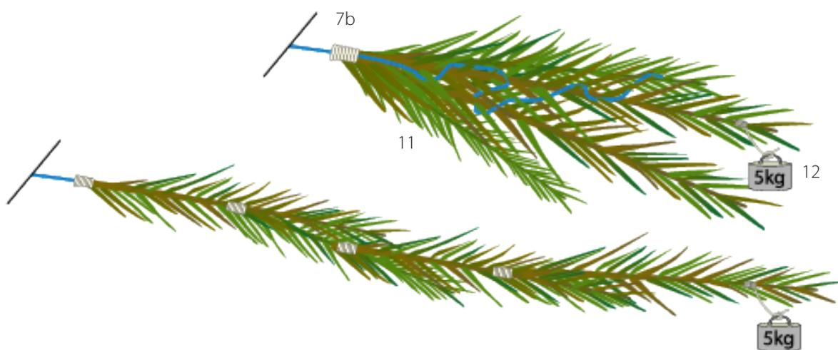
**Figure 21.** Diagram showing streamlined bamboo aggregators connected end-to-end in series (bottom) and bunched (top).
