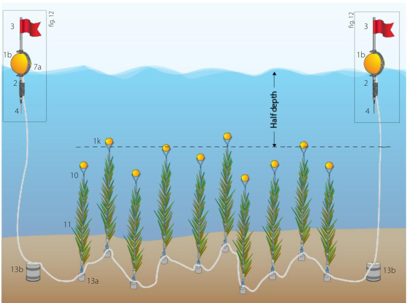
**Figure 3.** Modified lagoon FAD design showing the coconut fronds in a cluster.
