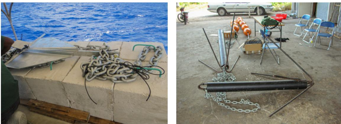
**Image 5.** A 25 kg danforth anchor (left) and a constructed grapnel anchor (right).
