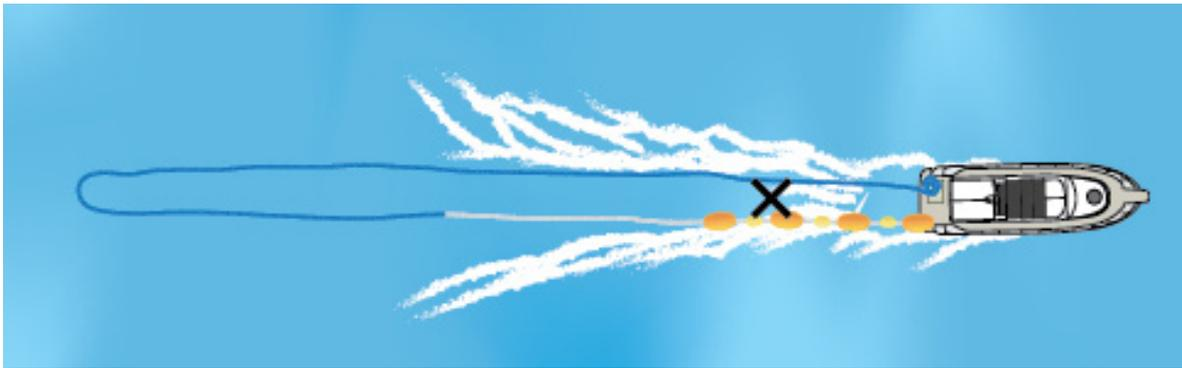
**Figure 33.** Sub-surface and lizard FAD deployment technique. The cross (X) represents the intended final anchor location.
