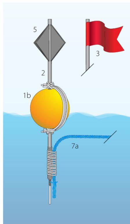
**Figure 12.** Diagram showing the rope connection to the flagpole.
