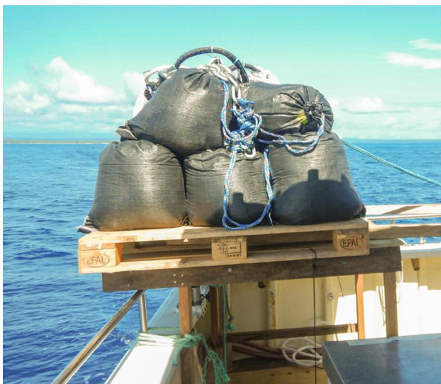
**Image 7.** Anchor constructed from sandbags.
