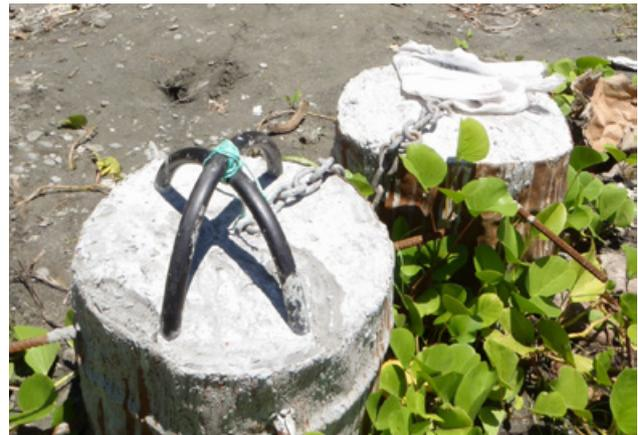
**Image 3.** Dual drum anchor showing the internal set-up (left) and prior to being deployed (right).
