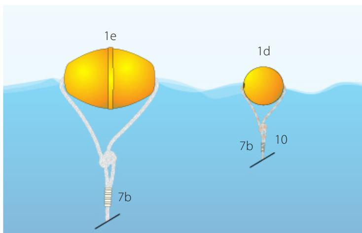
**Figure 15.** Diagram showing the end connection to a surface float with a centre hole.
