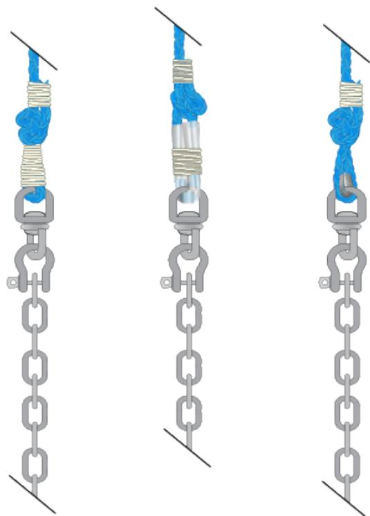
**Figure 29.** Anchor to main line rope connection.
