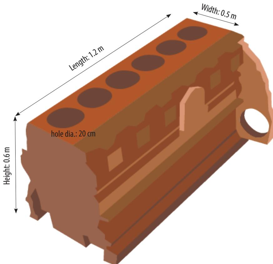
**Figure 27.** Example of calculating the volume of a recycled steel engine block anchor.
