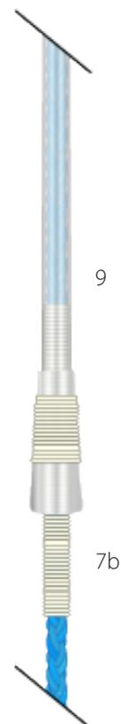
**Figure 19.** Diagram showing the binding onto the poly pipe sheath.
