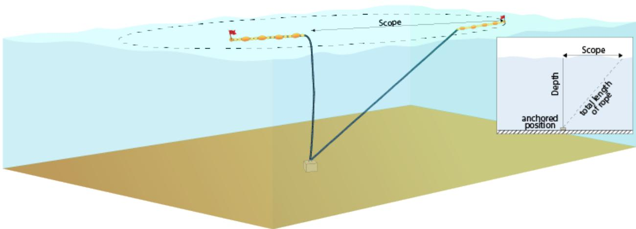
**Figure 26.** Diagram showing a FAD's scope.
