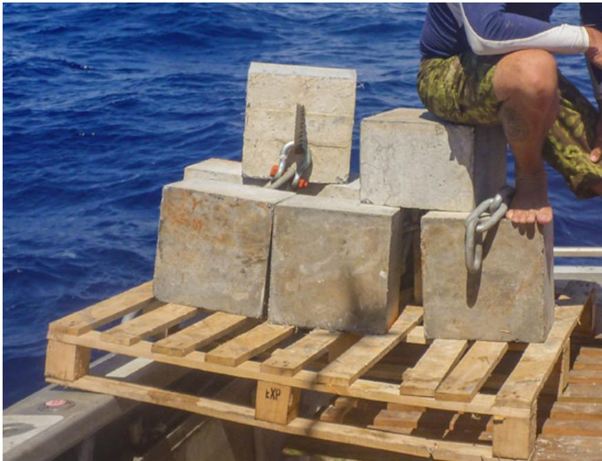
**Image 4.** Anchor deployment table on a small boat showing multiple small cement blocks attached in series.
