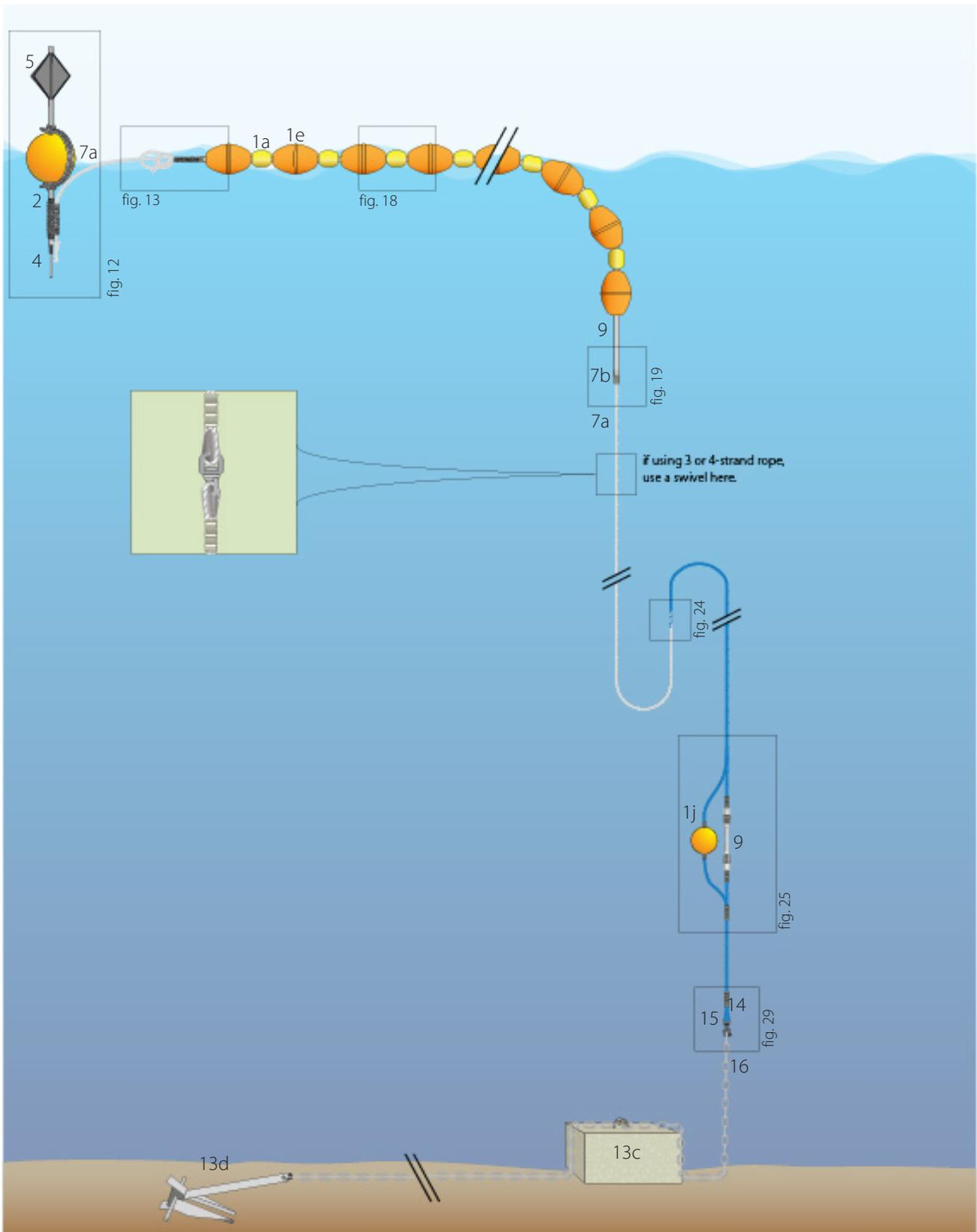
**Figure 6.** Indo-Pacific FAD design showing the upper floatation system used in offshore areas. More detail on the components in each of the boxed inserts can be found in section 4.
