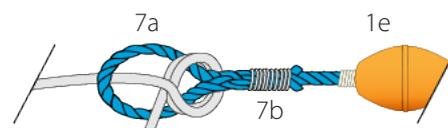
**Figure 13.** Diagram showing the end loop connection on the upper floatation.
