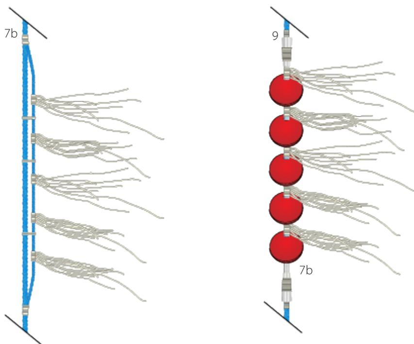
**Figure 20.** Diagram showing the attachment of aggregators using a secondary rope (left) and to the plastic tubing sheath on a sub-surface FAD (right).
