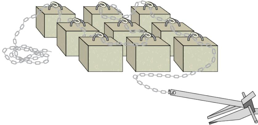
**Figure 28.** Diagrammatic representation on connecting multiple small blocks with galvanised chain.
