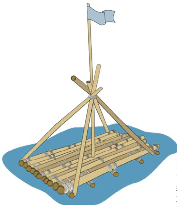
**Figure 5.** Large bamboo rafts are often used for the upper floatation of bamboo FADs, which can place greater stress on the mooring system and result in premature loss.
