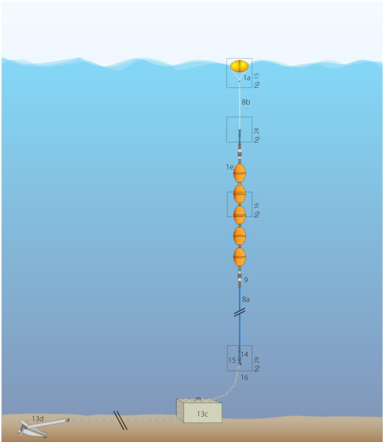
**Figure 7.** Subsurface FAD design showing the temporary surface marker to aid fishers to locate the FAD initially. More detail on the components in each of the boxed inserts can be found in section 4.
