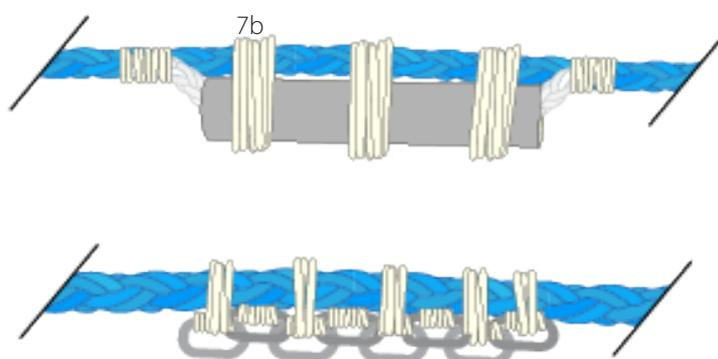
**Figure 22.** Diagram showing two counterweight options – cement tube (top) and galvanised chain (bottom) – and how they are rigged to the mooring line.
