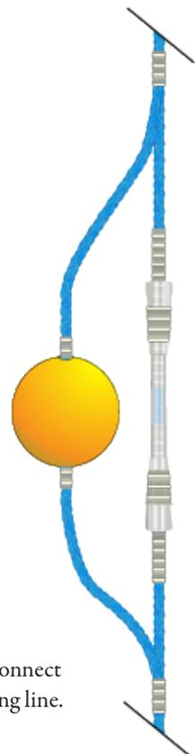
**Figure 25.** Diagram showing how to connect supplementary buoyancy to the mooring line.
