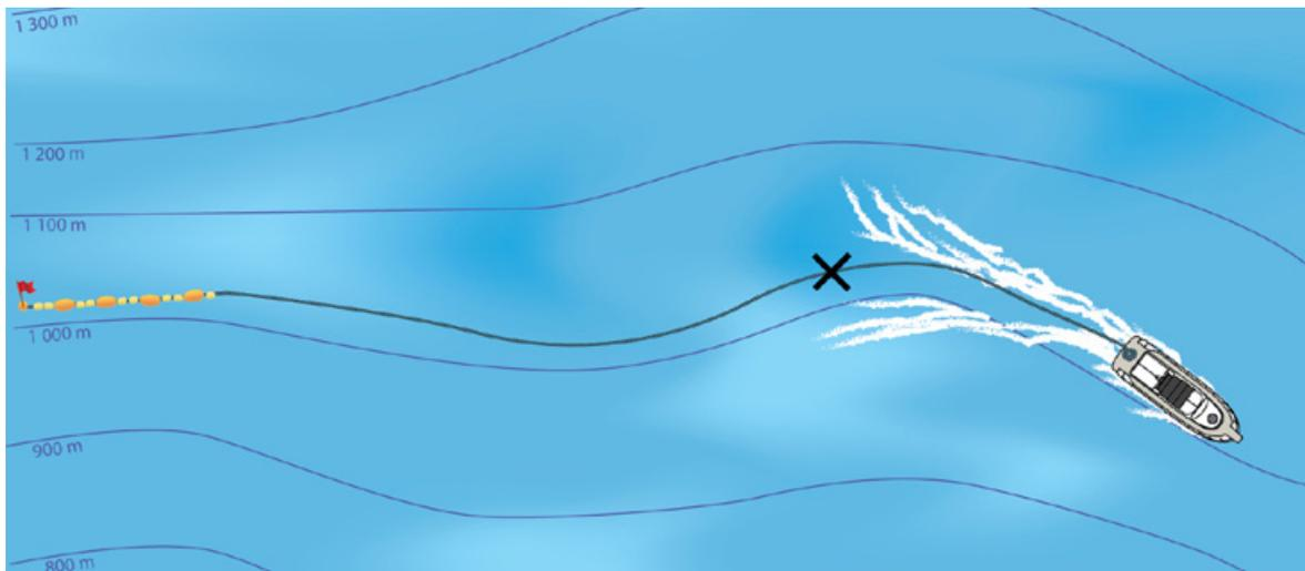
**Figure 32.** Straight line/contour deployment technique. The cross (X) represents the intended final anchor location.
