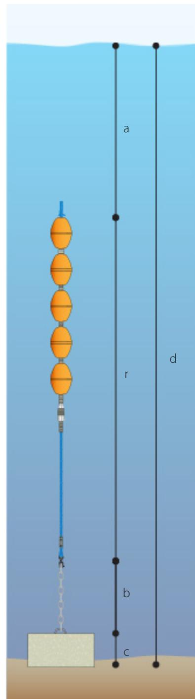
**Figure 23.** Diagram showing the components required for the calculation of subsurface main line rope length (a = floatation settling depth, b = chain length, c = block height, = deployment depth, r = main rope).
