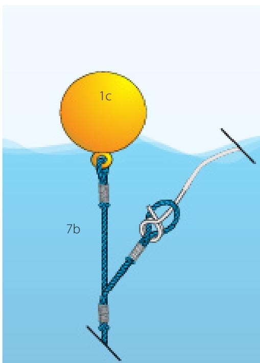
**Figure 14.** Diagram showing the detachable loop on the upper floatation for the bamboo FAD.
