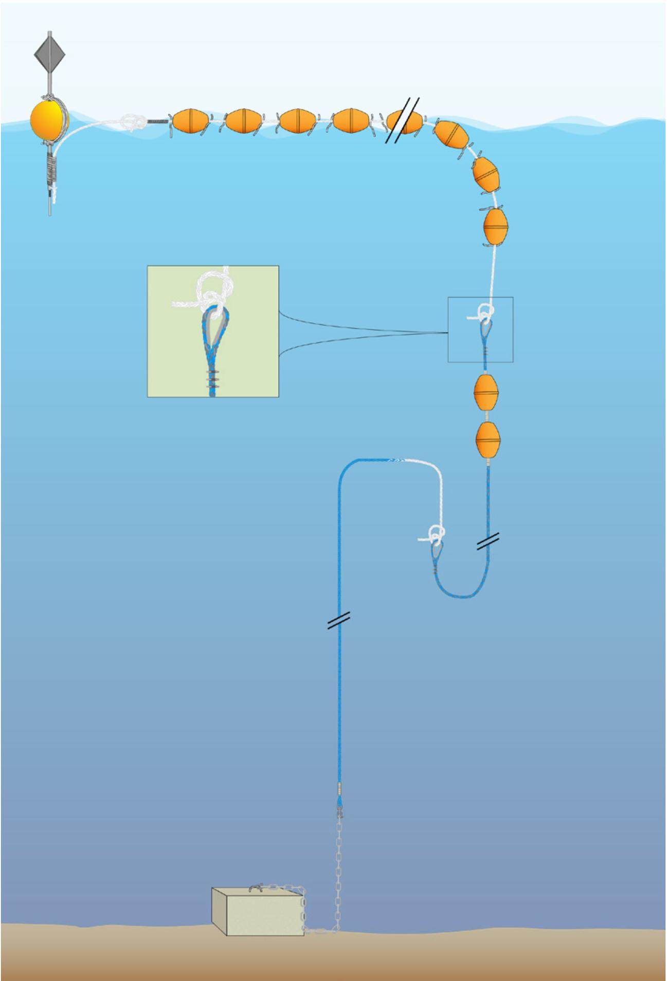
**Figure 10.** French Polynesia FAD design showing modifications.
