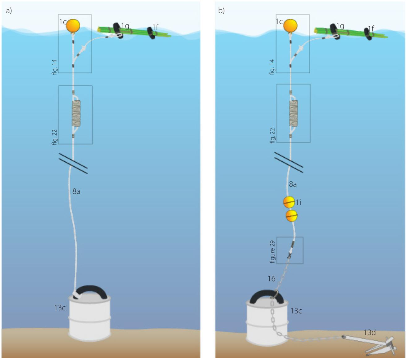
**Figure 4.** Bamboo FAD design showing: a) the basic version suitable for lagoons and bays; and b) the advanced version with additional anchor capacity being more suitable for nearshore environments. More detail on the components in each of the boxed inserts can be found in section 4.
