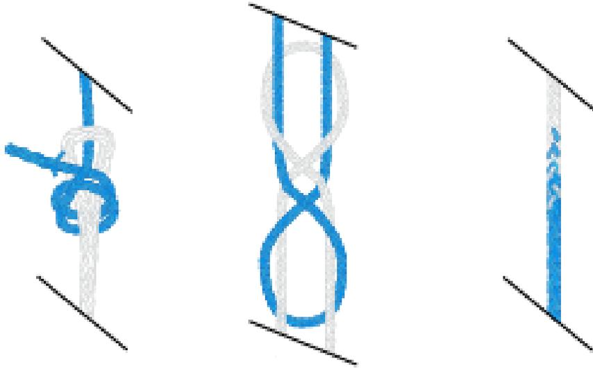
**Figure 24.** Diagram showing three options for connecting nylon and multistrand rope (left – double sheet bend; middle – monofilament carrick bend; right – splice).
