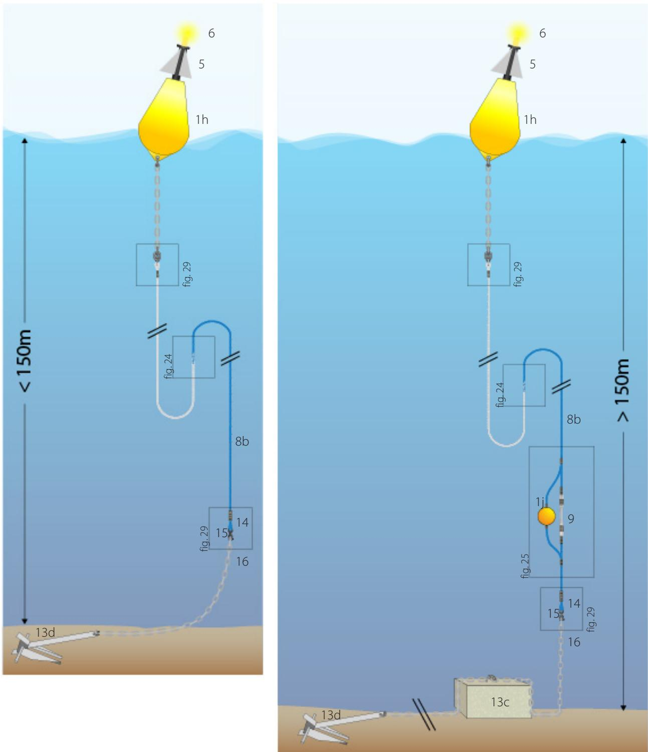
**Figure 9.** NSW DPI FAD design (left – NSW DPI design for shallow water; right – modified anchor system). More detail on the components in each of the boxed inserts can be found in section 4.
