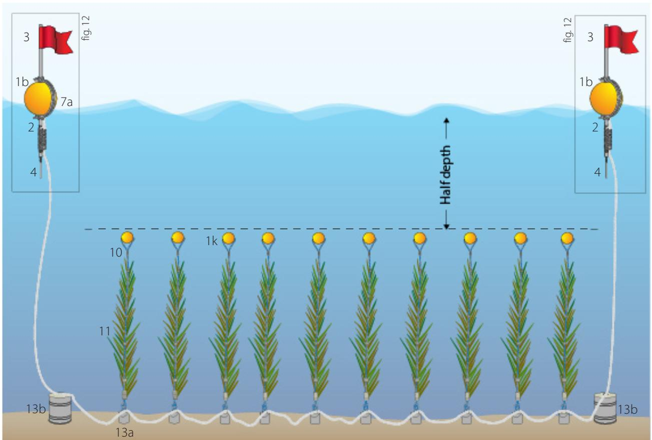
**Figure 2.** Lagoon FAD design showing the series of coconut fronds, with surface markers at either end.
