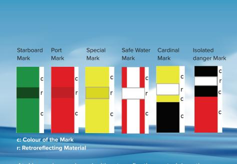
AtoNs can be equipped with retroreflective material, so the mariner can detect the position and colour at night by use of a searchlight
