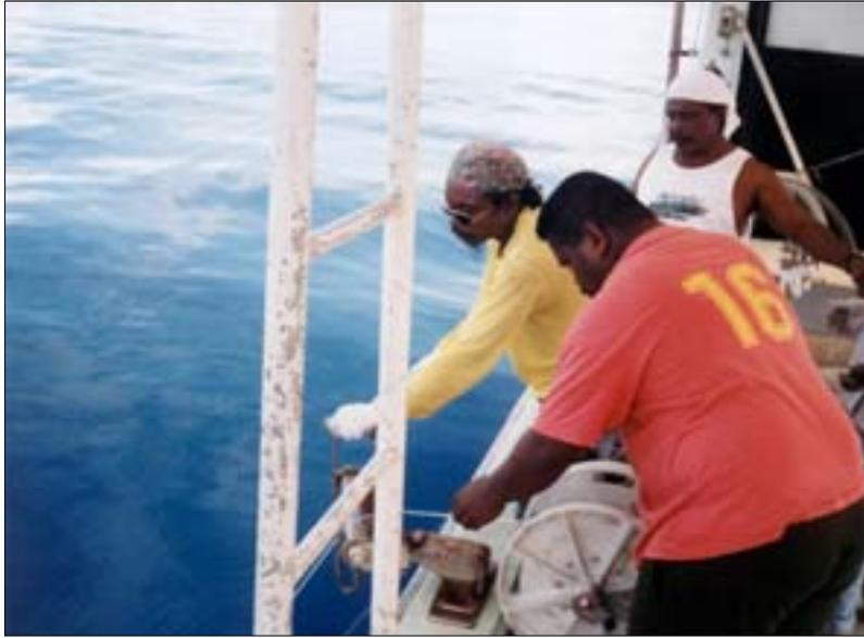
videotape on longline fishing, and a practical session on making up longline fishing gear. FV *Elechil* came equipped with a longline reel and monofilament gear, which were modified. Branchlines were shortened from 32 m to 15 m and new floatlines were made from tarred polyester line.
