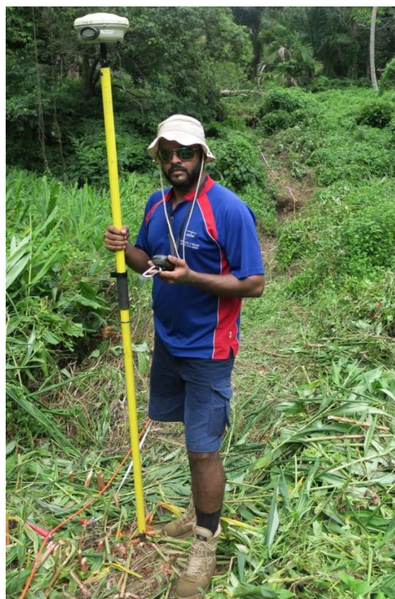
The Trimble R8 Rover unit mounted on a 2-m pole (Satellite Receiver).
