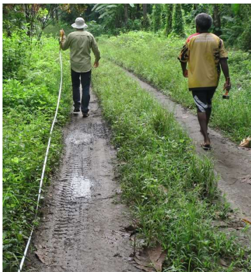
A measuring tape is laid out to mark the survey line.
