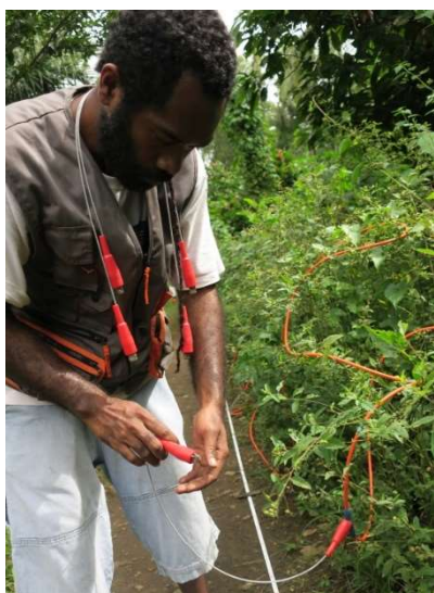
Securing electric cables to steel electrodes using connector cables.
