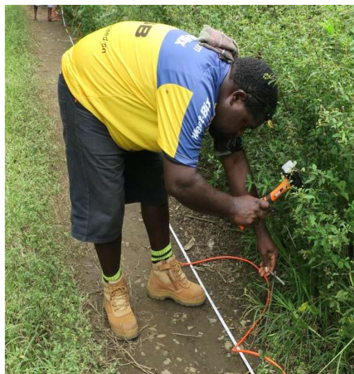
A hammer is used to ensure adequate ground contact of steel electrodes.
