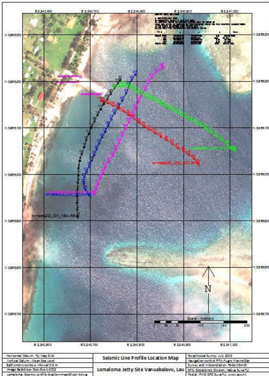
Figure 14: Seismic line track plot with respect to Lomaloma Jetty.
