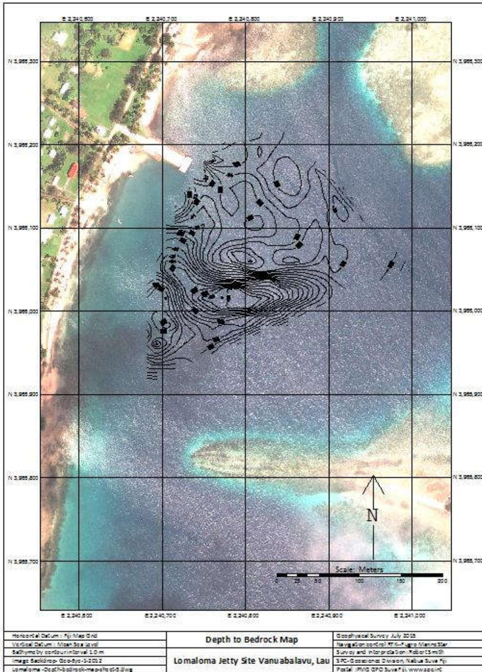
Figure 18: Top of bedrock as interpreted from the seismic data. The contours are referenced to MSL with a contour interval of 1.0 m.
