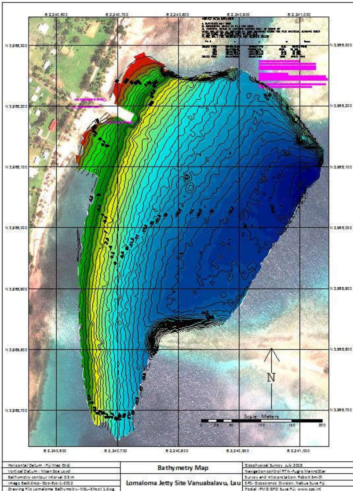
Figure 8: Detail of the bathymetry around Lomaloma Jetty. Contours interval is 0.5 m. The bathymetry reflects a very uniform slope and curvature setting. Minor scouring can be interpreted from the contours close to the southern end of the jetty. This is probably due to the fact that vessels prefer approaching from the south to dock at the wharf.
