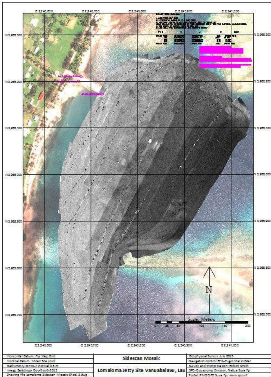
Figure 11: Sidescan mosaic compiled from the multibeam data. Reef structures are clearly identifiable from the sediments of the basin and offshore areas. Different shades of grey in the sediments represent different sediment types and some artefacts of gain control during acquisition.
