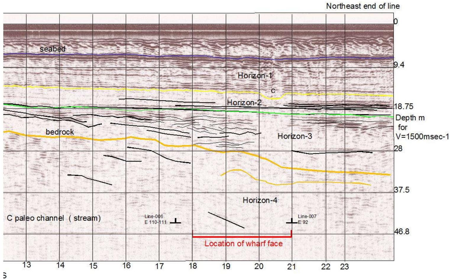
Figure 16: Detail of the seismic reflection patterns in the cross section at the wharf face.
