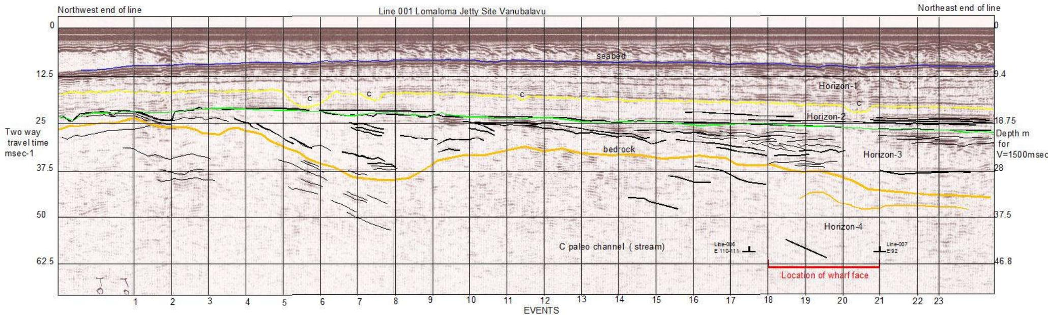
Figure 15: Interpretation of single channel seismic profile Line LOM\_seis\_202\_001.15554.raw
