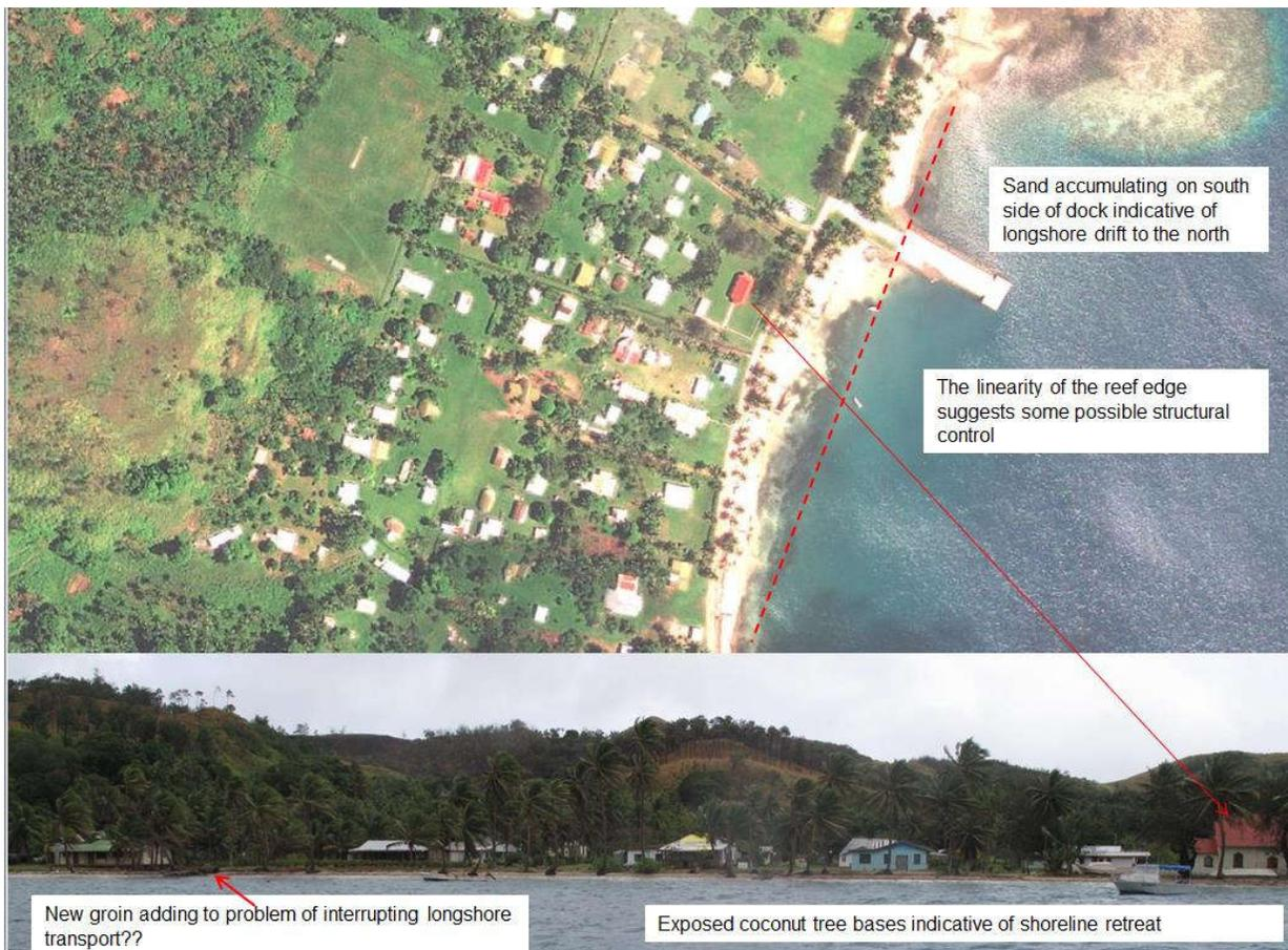
Figure 13: Shoreline erosion south of the jetty head. In the Geoeye-1 image of 2012 there is more sand accumulated on the south side of the jetty (North is page up) indicative of northward transport system. Large cusped erosion scars are also apparent with underlying reef (beachrock?) exposed.
