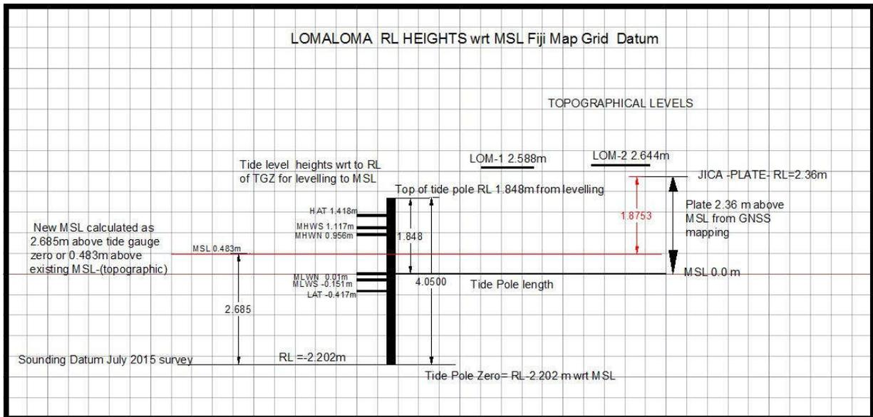
Figure 6: AutoCAD schematic depicting the relationship between the heights of the various Tide Datums, Mean Sea Level (MSL) and the control bench marks.
