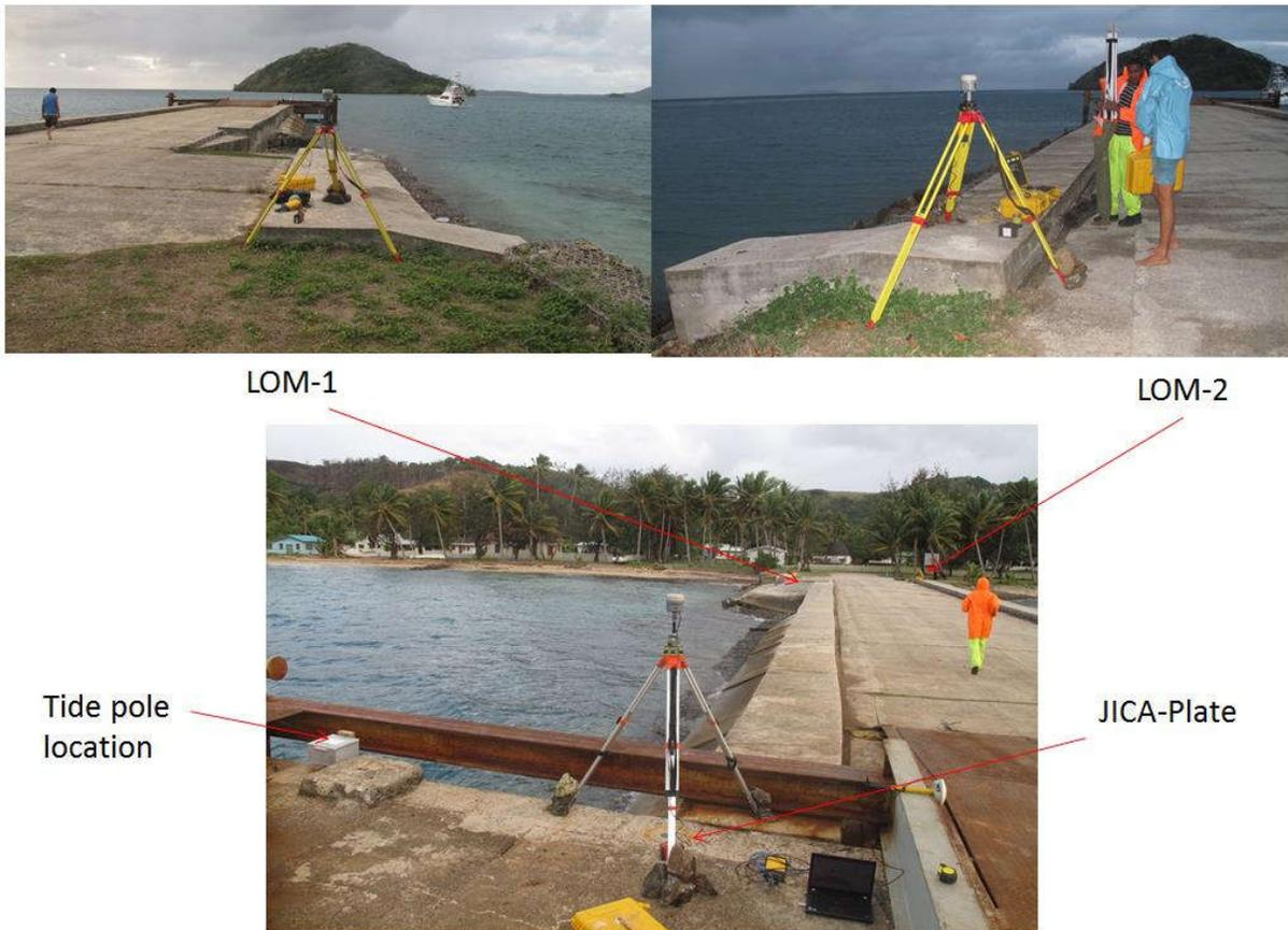
*Figure 4. Photo diagrams showing the control points surveyed using GNSS positioning and post processing of data to determine positions and elevations with respect to the Fiji Map Grid. This data are contained in AutoCAD dwg files in the data disc in Appendix 8.*
