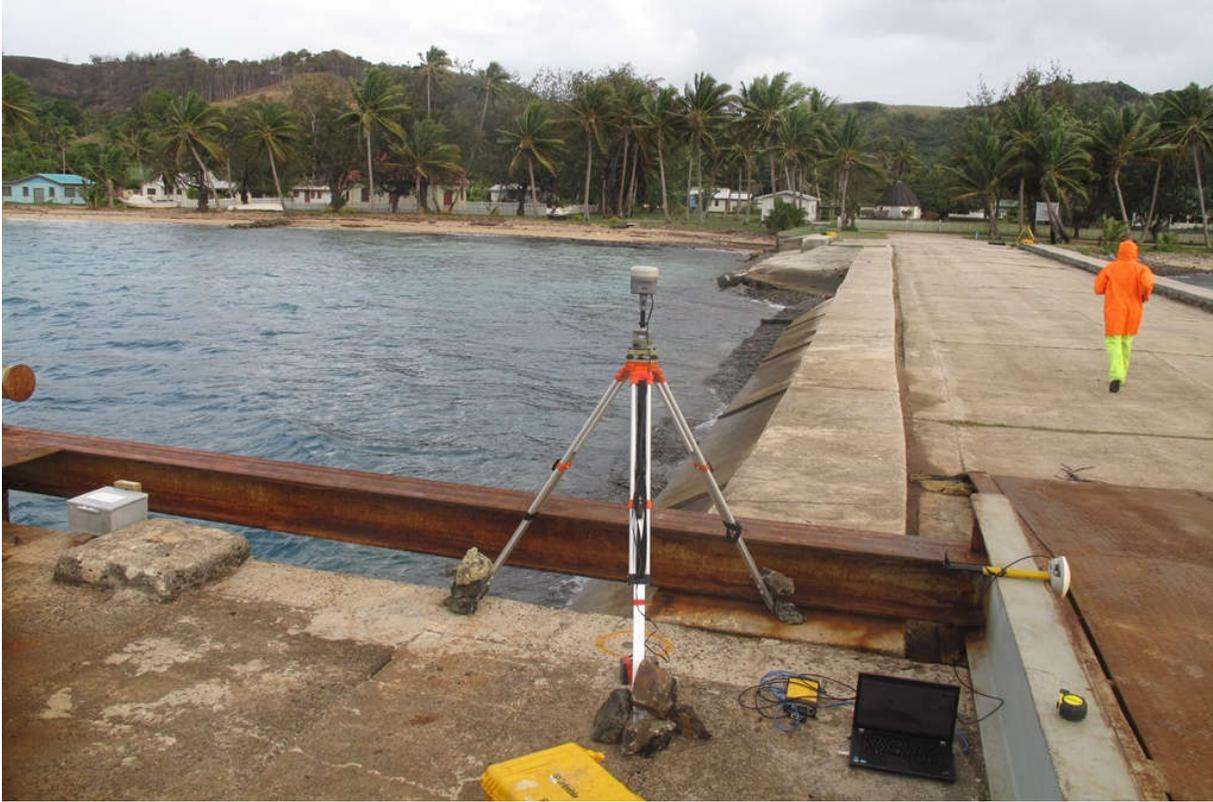
*Plate 1: GNSS Net R9 recording on location at the “JICA-PIN” brass plate.*
