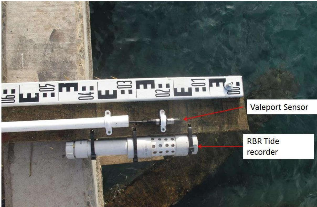
*Figure 3: Tide gauge sensor setup showing the actual position of the sensors with respect to the tide pole. Both were placed at 0.2 m above the zero point of the tide pole.*
