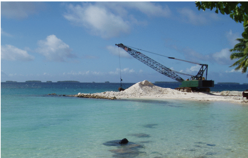
Figure 5. Shoreline based hydraulic excavator extracting sand and gravel from the Majuro Lagoon.
