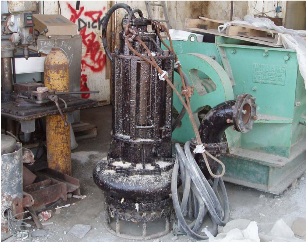
Figure 6. Suction dredge pump to extract sand and gravel from the lagoon bed.
