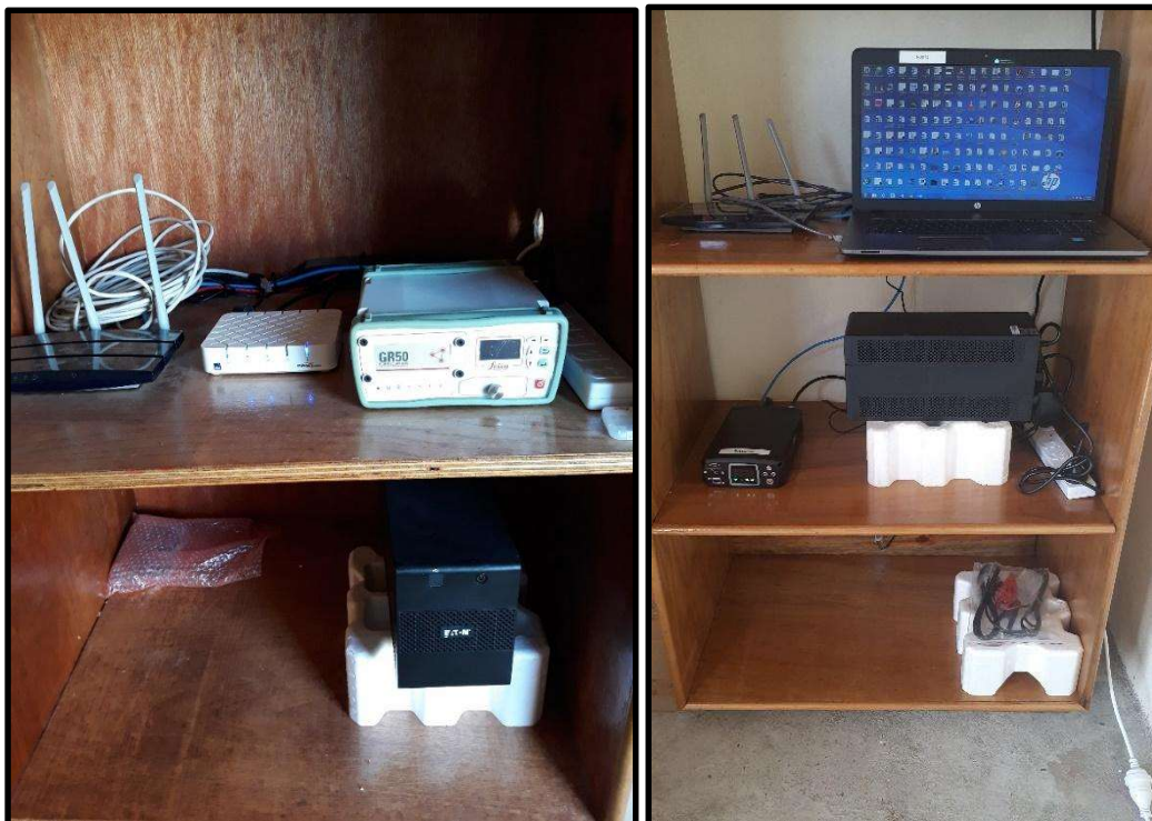
Figure 9: inside the GNSS CORS hut, typical set-up of the GNSS receiver with the internet router and the UPS.
