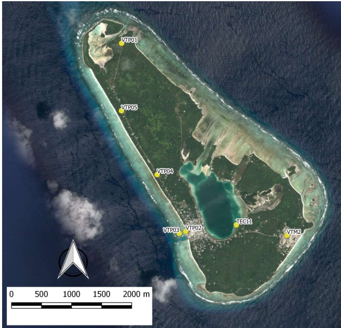
Figure 9: Location of benchmarks established as part of the survey. Benchmark elevation corrected from the continuous GPS (CGPS), TUVA based in Funafuti. Source: Google Earth 2015
