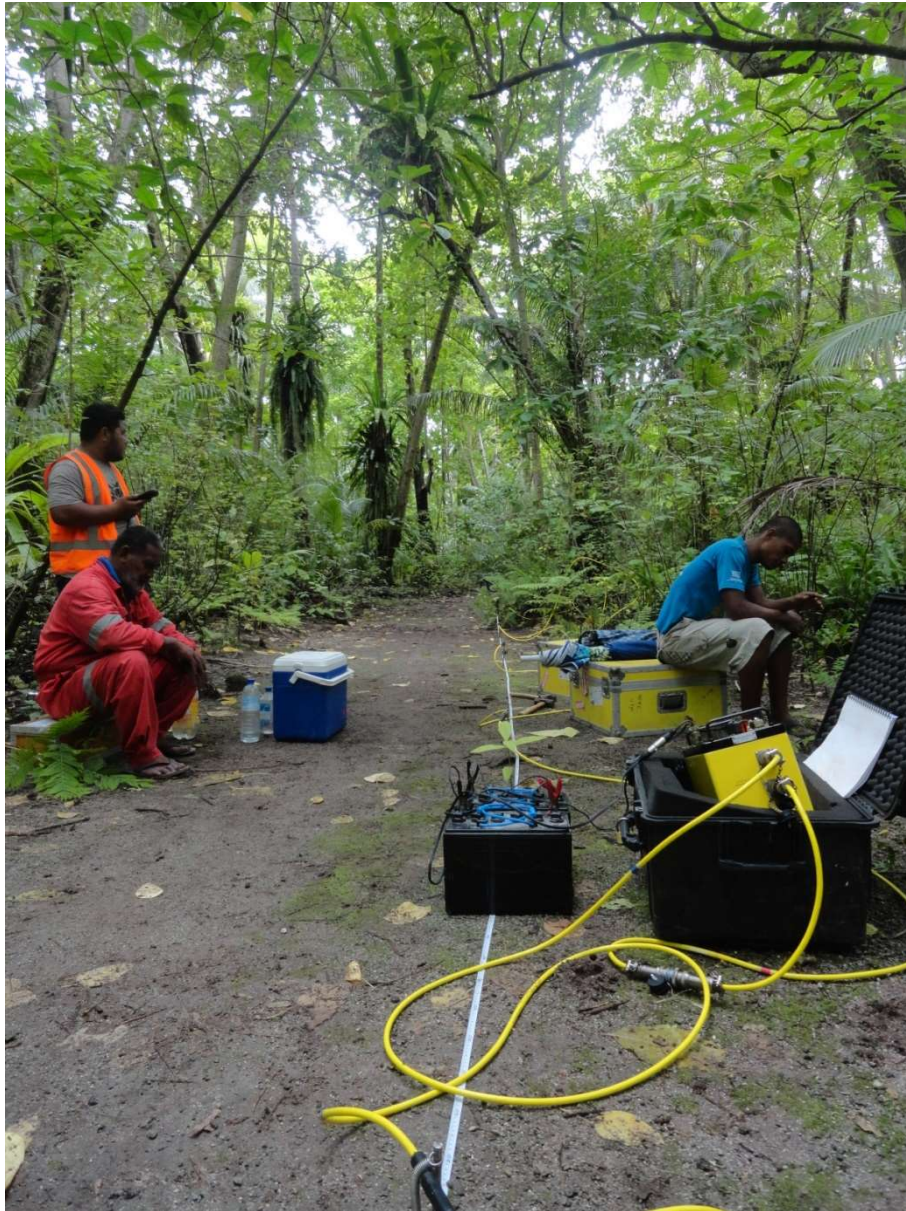
Figure 20: The resistivity survey lines along established tracks on Vaitupu.
