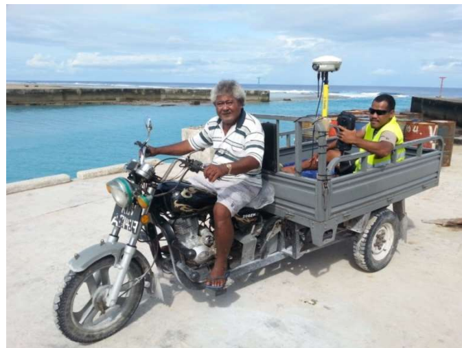
Figure 11: Continuous mode of RTK survey with the rover mounted on a trailer pulled by a motorbike.
